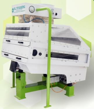
Vibro Destoner machine workes based on the difference in grain specific gravity, grainsize, shape and surface state. The working table is covered with a woven wire mesh bed, through which air flows from below.
