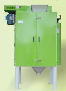
It is an advanced quality machine specially designed for splitting different types of pulses, grains and spices like Red Lentil (Massor), Black Lentil (Urad), Bean Lentil (Moong), Chikpea (Chana), Toor (Arhar), Coriander (Dhaniya) etc. It is also used in plucking the mustache of Cumin, Fennel, Ajwain etc. A very important machine for any type of pulses, grains, and spice mill to ensure minimum loss and maximum production.
