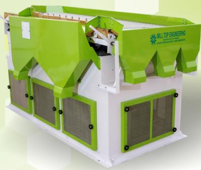
Gravity Separator is used for separating grains of the same size but with different specific weight, it is used effectively for removing partially eaten immature & broken seeds to ensure maximum quality of the product. Gravity Dack rpm is controlled by automatic v.f.d. system.
